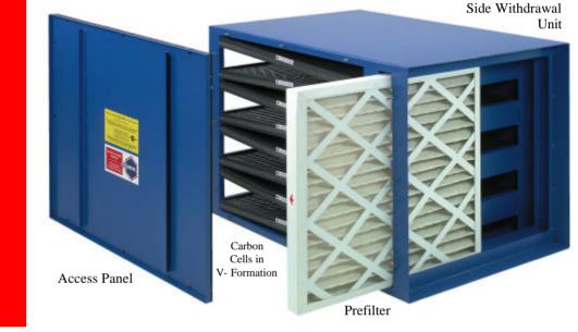
The prime use of the Activ-V filter is a recirculation filter in air conditioning and ventilation systems for the purpose of removing the odour and staleness associated with the recirculation of conditioned air. It is also suitable for the removal of light concentrations of specific chemical and gaseous contaminants from industrial intake or exhaust systems.
