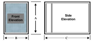
Minimum Carbon Weight Loading: 80kg/1.0m³/sec. Resistance to airflow: 110 Pa excluding prefilter
