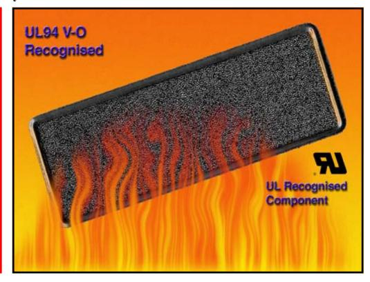
The unique construction of this filter, with strong corrosion resistant wire frame thermoplastically encased and heat bonded to flame retardant media, provides the flexibility to produce the filter in virtually any required size or shape. The post treated, polyurethane, open cell foam media is available in a variety of porosities and thicknesses, all displaying excellent dust holding capabilities when compared to equivalent metal mesh or disposable filters.
