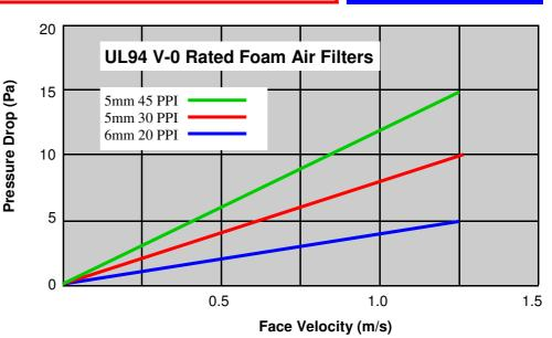
As the filter becomes laden with dust the initial pressure loss will increase. The final recommended resistance is reached when the initial pressure drop has increased by 65 Pascals. The arrestance efficiency of 65% EU2 is based on the filters ability to hold synthetic dust by weight, the test dust particle size ranges from 0-80 microns. The filter efficiency will peak at 1 m/sec, with a reduction likely to be seen when operated above this.
